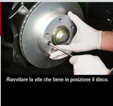
Re-fasten the screw which keeps the disk in position.
