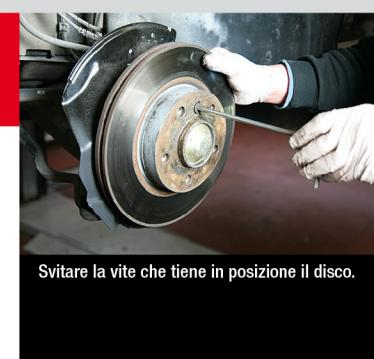
Unfasten the screw which secures the disk in position.
