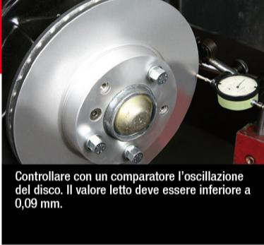
Using a comparator, check disk oscillation. The read value must be less than 0.09 mm.
