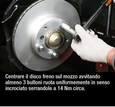
Centre the brake disk on the hub, screwing at least 3 wheel bolts uniformly in crossed direction, tightening them to about 14 Nm.
