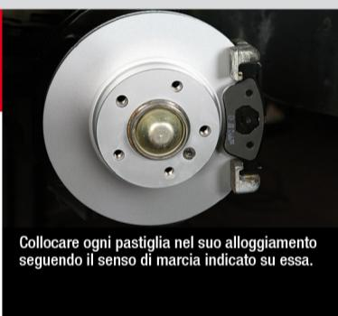
Fit each pad in its seat, following the direction indicated on the pad.
