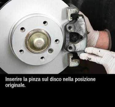
Fit the caliper on the disk in its original position.
