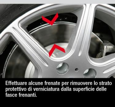
Brake a few times to remove the protective paint layer from the surface of the braking strips.
