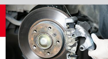
Withdraw the body of the caliper, complete with internal pad, without disconnecting it from the brake system pipes.
