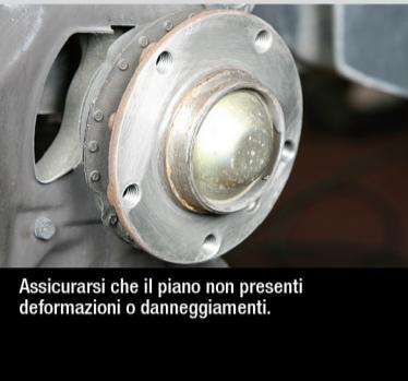
Make sure that the surface is not deformed or damaged.
