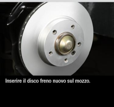
Fit the new disk brake on the hub.
