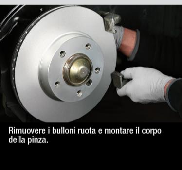
Remove the wheel bolts and install the caliper body.
