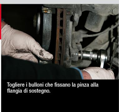
Remove the bolts which secure the caliper to the support flange.
