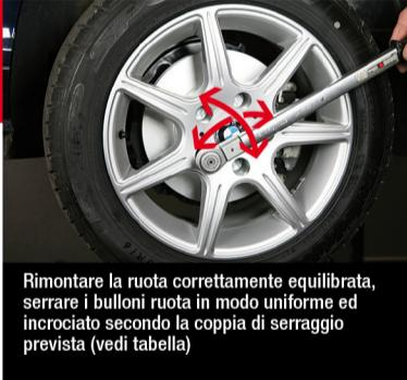
Re-install the correctly calibrated wheel, cross-tighten the wheel bolts uniformly according to the specified tightness torque (see table).
