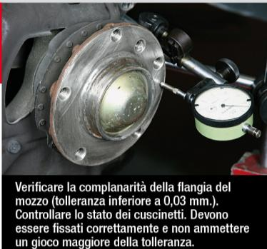
Check if the hub flange is on the same plane (tolerance of less than 0.03 mm). Check the condition of the bearings. They must be correctly fixed and must not allow play greater than tolerance.
