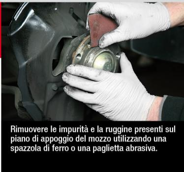
Remove dirt and rust from the support surface, using a steel brush or abrasive steel wool.
